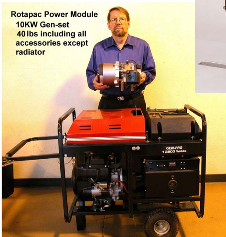
The Rotapac 10 KW generator being held by Paul is shown as a comparison to the 13.5 KW generator from Gillette (weight is 350 lbs)
